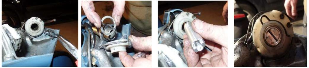
Fasten the torque support with the headlight so that it is tension-free.
