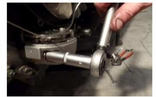
Shorten the bowden cables and cover the selector box and reassemble the handlebar.
