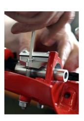
The pump must sit in the middle of the throttle guide.
