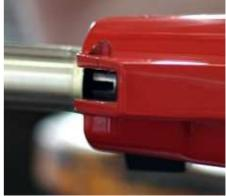
With the pliers push the push rod slightly into the pump, insert the brake lever and then tighten it correctly.
