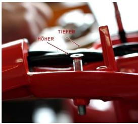
Mount the pump and tighten it with a Screw on the front stud.
