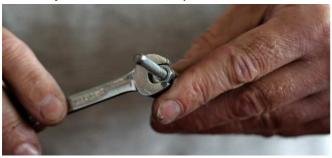
Unscrew M5 bolts and remove pump; the studs remain in the handlebar.
