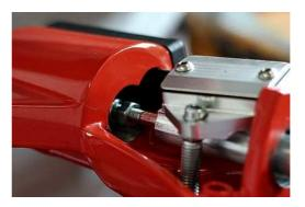
Carefully remove lever and push rod and fix with the nut in the length.
