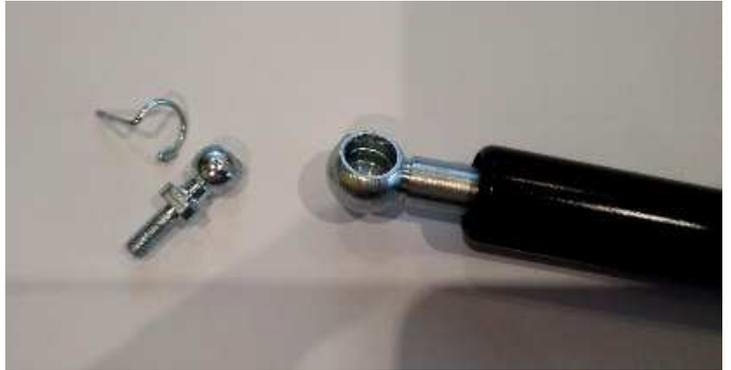
2. Screw the two balls in the holes of the plate with two washers next to the ball and one next to the nut.
