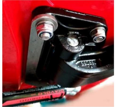
4. Insert the right spring with the thinner part from the left side into the right ear of the center stand, using one washer left and right. After that do the same with the other spring.
