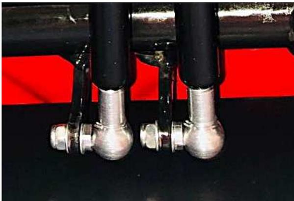
5. Push the springs back onto the balls until they latch, then fix them with the splints.
